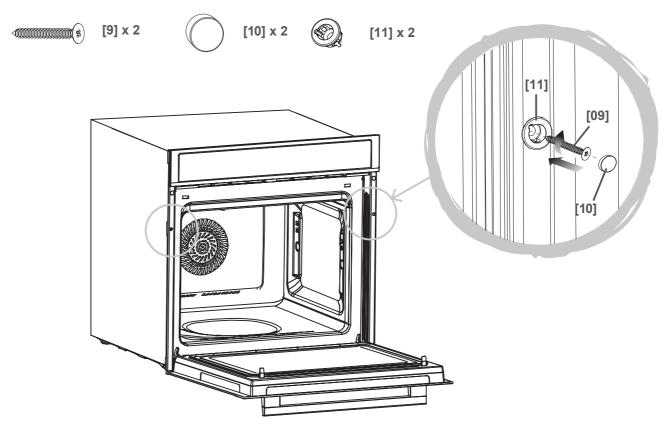
Once the oven has been lifted into place inside the appliance housing, locate the two holes in the casing of the oven and fix it into place using [09], [10] and [11].
