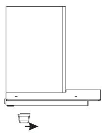
2. The filter/grill has been fixed onto the hood with 2 screws. Kindly unscrew the filter/grill. Take out the filter/grill by 20 dgree(as picture).
